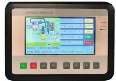
LX series System Management Control Panel
